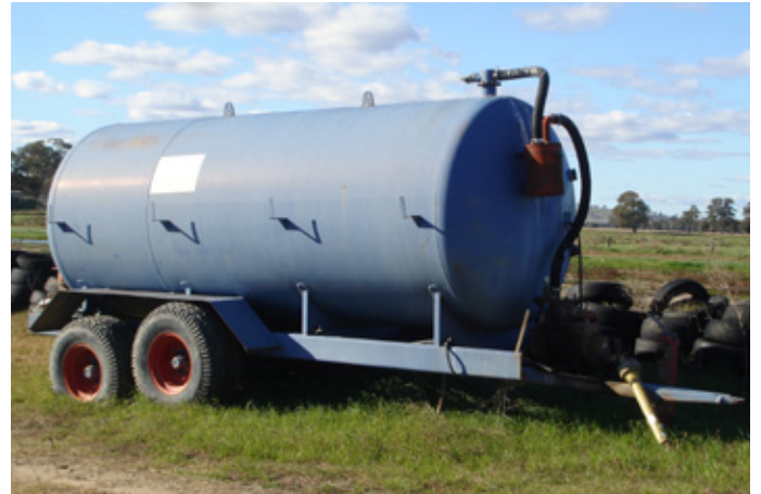
The effluent tanker is used to spray treated effluent onto pastures - with visible results
