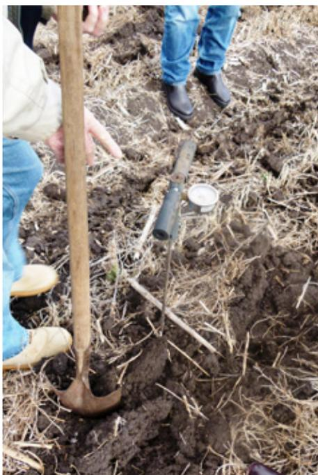
*A penetrometer test shows deep, friable soil*
